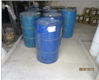
External photo(s) of the production unit(s) 7-7 Missing secondary container.JPG
